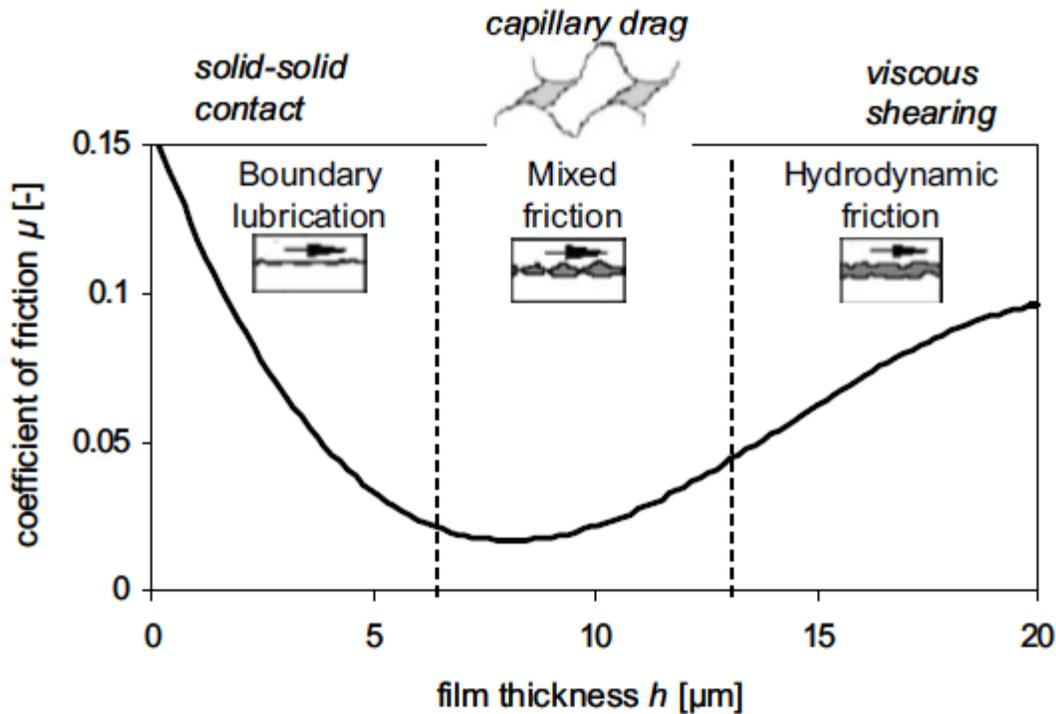
Figure 1. Coefficient of friction of ice as it varies with film thickness. The liquid film on ice ceases to exist at approximately  $-200^{\circ}\text{C}$ . As the ice temperature approaches this point, the thickness of this film decreases and the coefficient of friction is affected in a non-linear manner (Kietzig, 2010).
