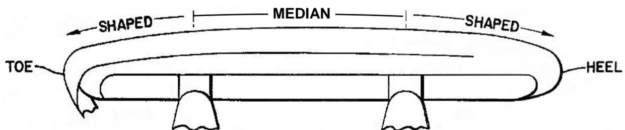
Figure 2. Profile of ice hockey skate blade. From left to right, the blade comprises a shaped toe, median section, and shaped heel. The median section is the portion that is sharpened to match the radius of curvature. The point of tangency is not restricted to this boundary; it can be located anywhere from the shaped toe to the shaped heel (adapted from U.S. Patent No. 4,907,813, 1990).
