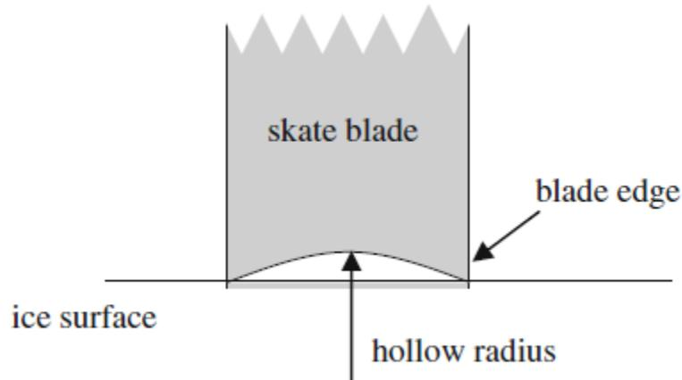
Figure 3. Diagram of ice skate blade showing hollow radius. The radius of hollow of the skate blade determines how deep the blade will cut into the ice. A smaller radius will cause the blade to dig deeper into the ice; a larger radius will not cut as deep (Federolf and Redmond, 2010).
